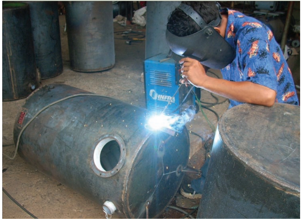
A sand filter for an irrigation system is welded at Vásquez Mecanizaciones in Honduras.
