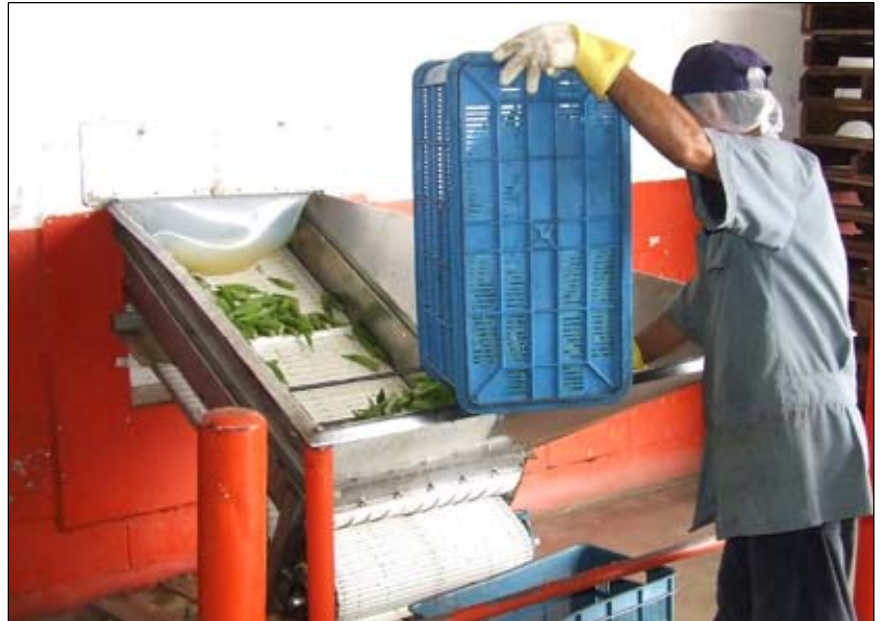
To minimize cross-contamination, okra from the field is unloaded outside the processing facility and put on a conveyor belt for a pre-washing.
