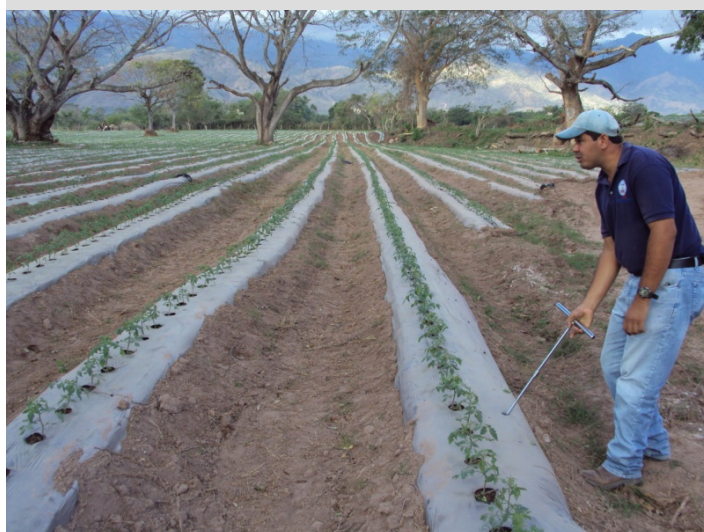
Soil core sampler used to measure soil humidity, Comayagua
